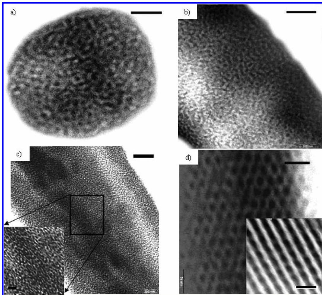
**Figure 2.** TEM images of IS29 system: (a) cross section of fibers spun from 30 wt % solution in THF, scale bar = 100 nm; (b) along the axis of as-spun fiber, scale bar = 200 nm; (c) along the axis of fiber annealed for 24 h at 80 °C, scale bar = 200 nm, inset scale bar = 50 nm; and (d) film cast from 10 wt % solution in THF, side view and top view scale bars = 50 nm.
