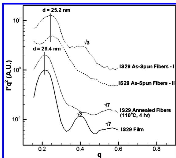
**Figure 3.** SAXS patterns of IS29 fibers and film. Fibers were spun using a 30 wt % solution in THF. Two different SAXS curves for as-spun IS29 fibers taken at different regions of the same sample are shown.
