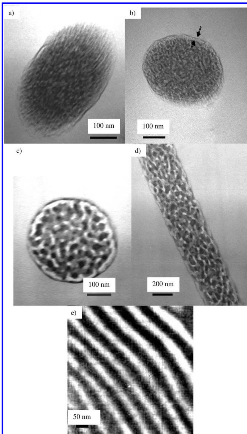
**Figure 4.** TEM images of IS53 copolymer: (a, b) two cross sections with different domain structures of fiber spun from 25 wt % solution in THF; (c) cross section of fiber annealed at 90 °C for 12 h; (d) along the axis of fiber annealed at 90 °C for 12 h; (e) film cast from 10 wt % solution in THF.
